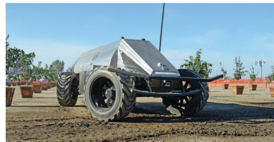
An operator using a computer tablet can control up to eight GUSS self-propelled autonomous sprayers at once. At the World Ag Expo demonstration pictured here, a GUSS airblast sprayer navigates a mock orchard.
