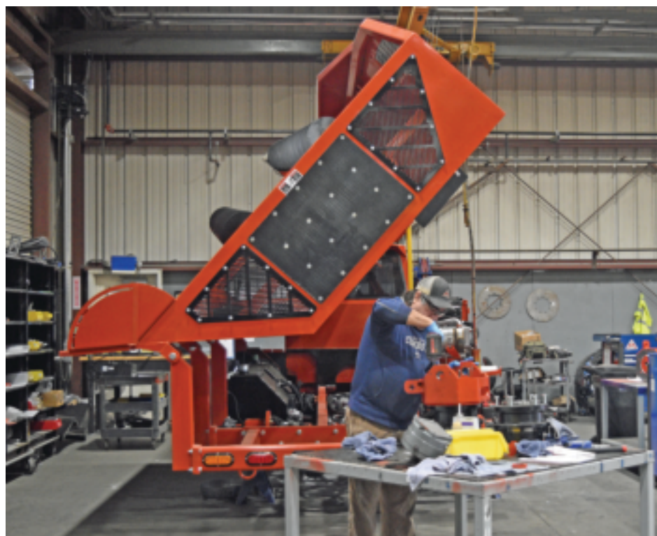
A machinist torques nuts on a machine part-way through manufacturing.
