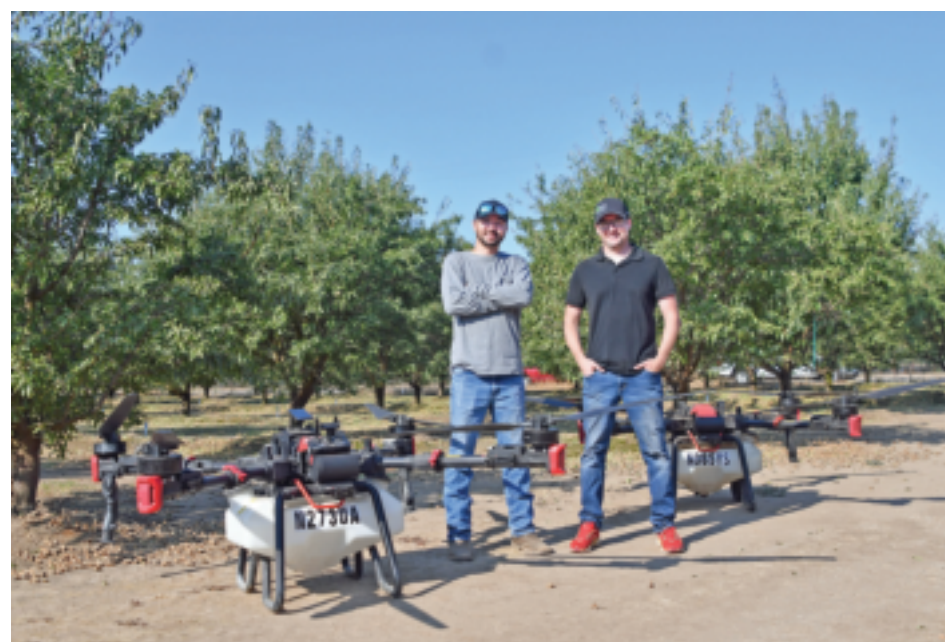
Brandon Steed (left) and brother Nicholas are both licensed to fly agricultural spray drones. Each of the XAG Pro 100s that they fly weighs more than 100 pounds empty.
